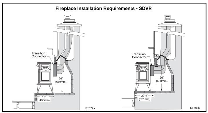
Fig. 38 SDVR minimum lintel height for flush or forward placement.
